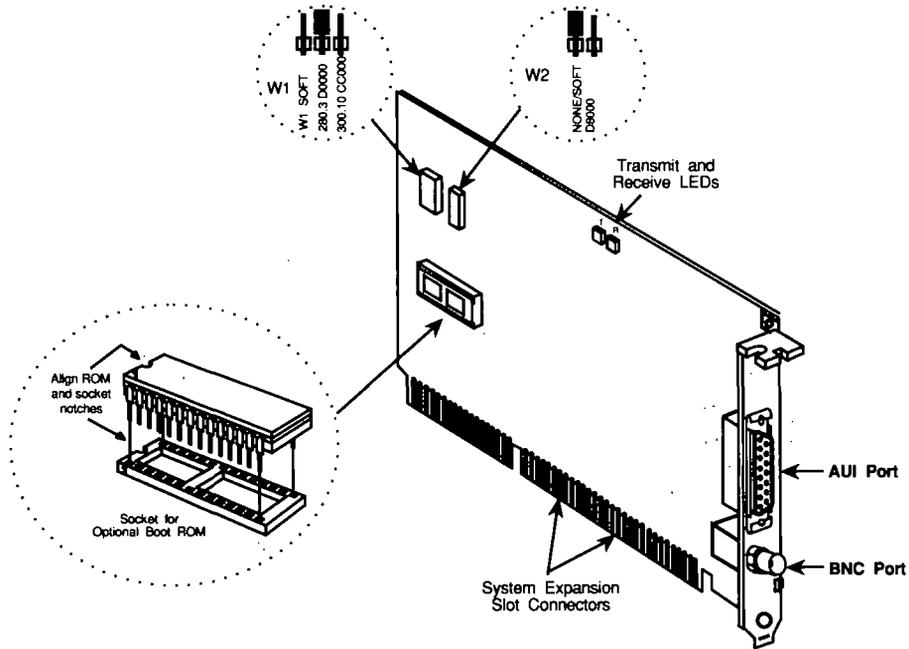
Figure 1. Ethernet Elite16 Adapter
