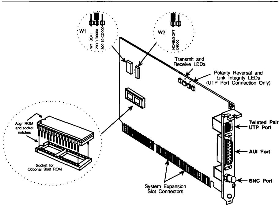
Figure 3. Ethernet Elite16 Combo Adapter
