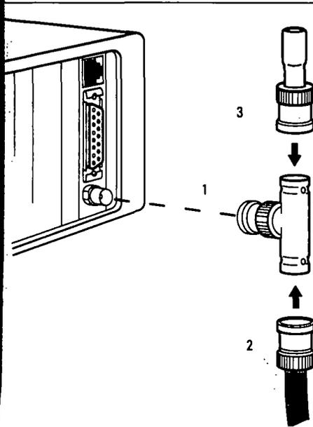
**Figure 14. Attaching the T-Connector, Cable & Terminator**
