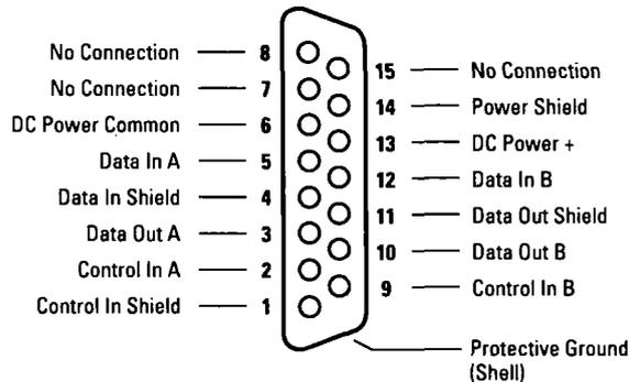
Figure A-1. Male AUI Connector Pin Functions
