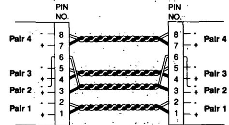
**Figure 18. Interface Cable Wiring**
