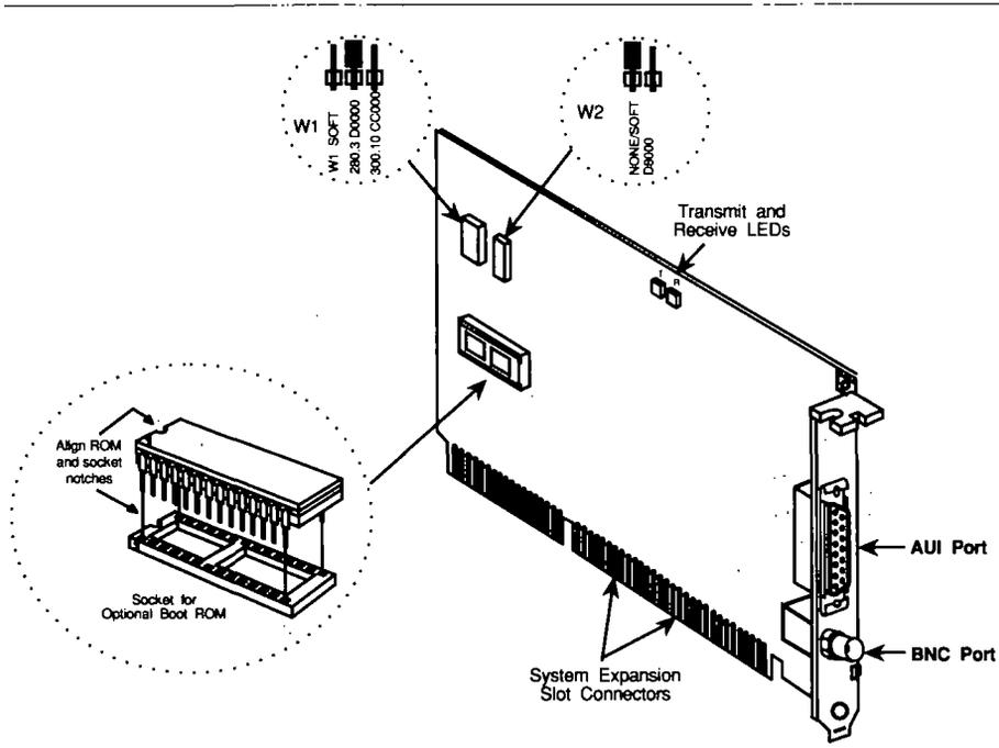
Figure 1. Ethernet Elite16 Adapter
